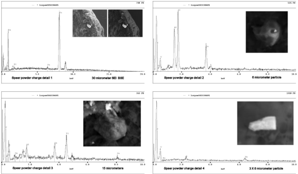
FIG. 11—Speer Lawman powder charge metal embeds with spectra.
