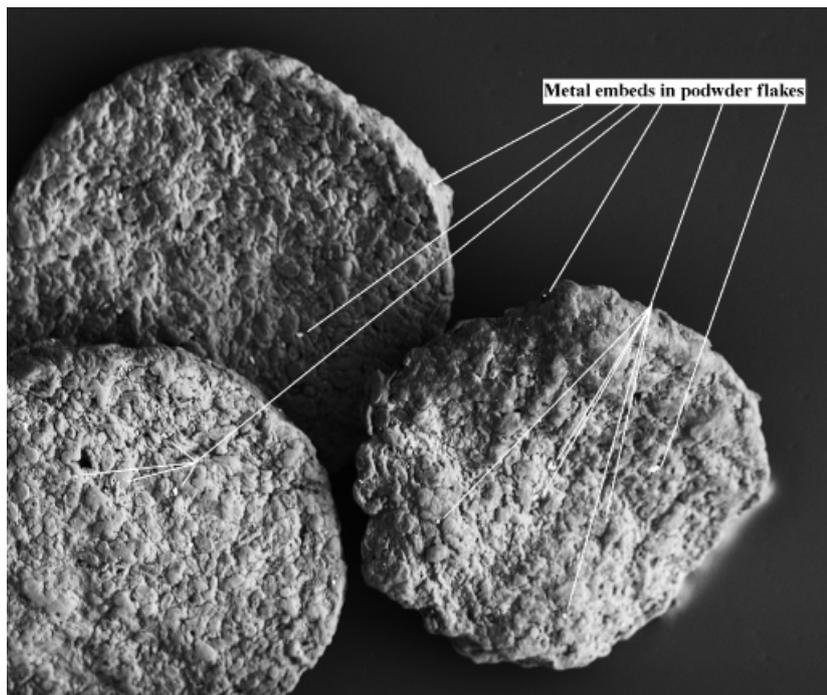
FIG. 10—Speer Lawman CleanFire™ powder flakes with metal inclusions indicated.
